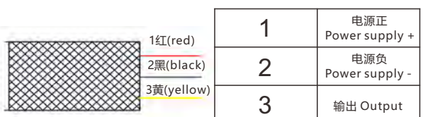
PTC-1200, PTC-1300, PTC-138, PTC-40B, PTC-40F, PTC-40HA电压型接线图 Voltage type wiring diagram
